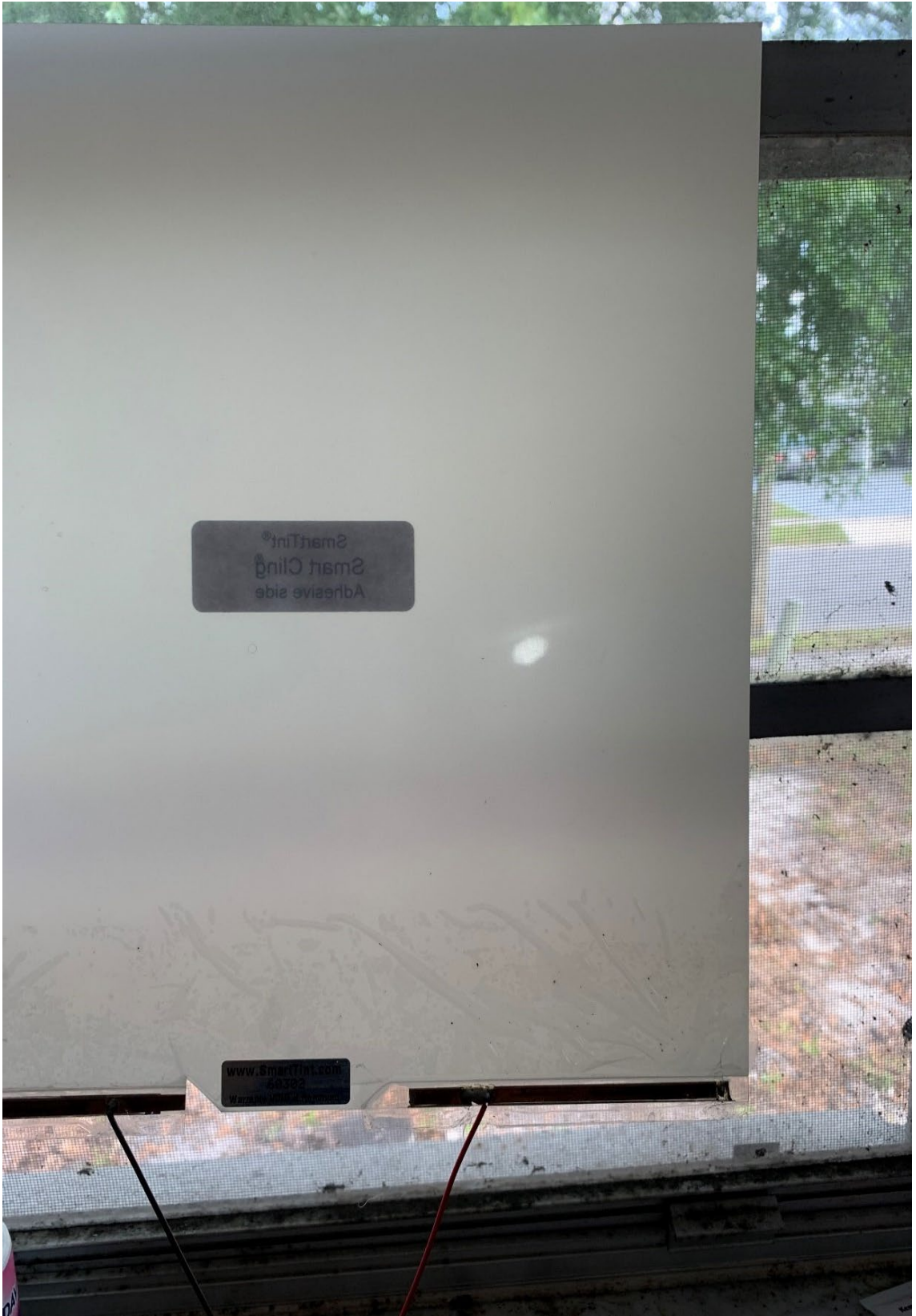
Figure 38: Smart Film (PDLC) in OFF state
