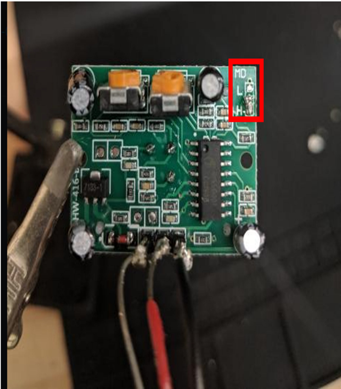
Figure 37: PIR sensor (Jumper missing - solder to activate repeatable trigger mode)
