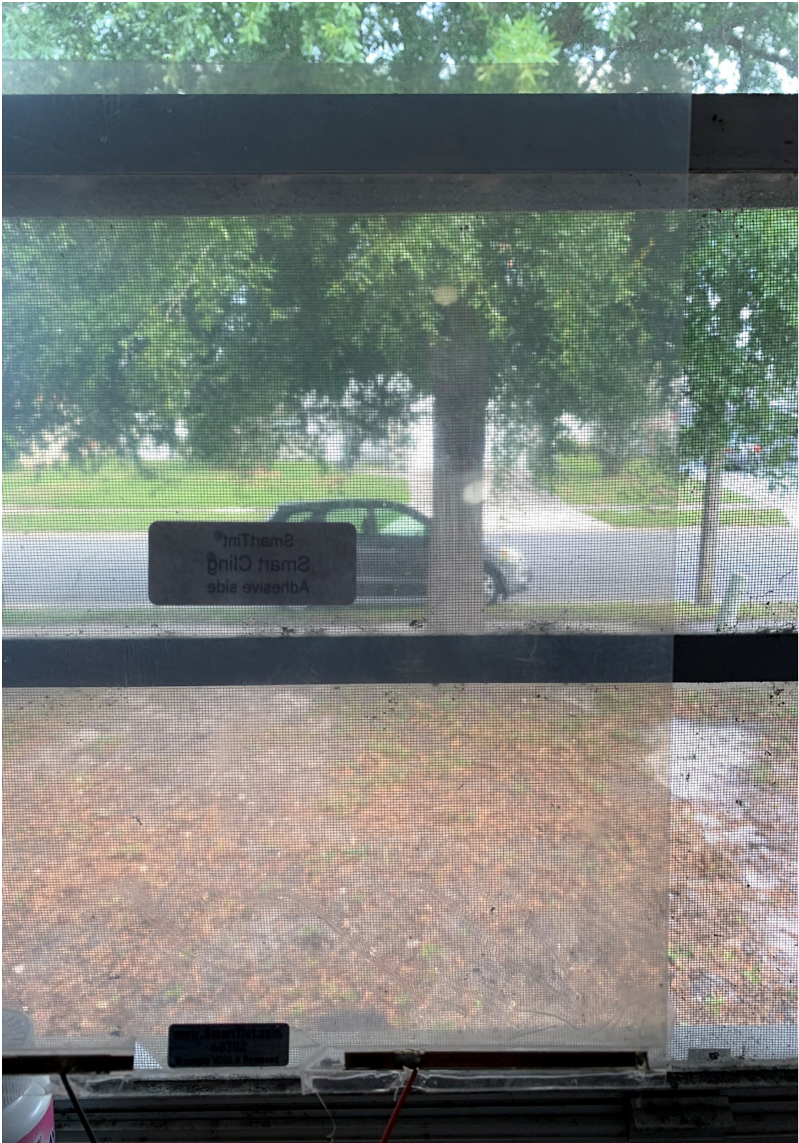
Figure 39: Smart Film (PDLC) in ON state
