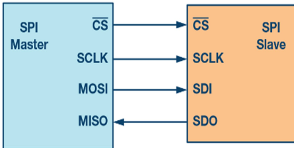
Figure 25: Basic SPI single Master and Single Slave configuration
